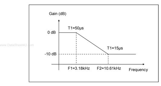
The filter response scales with sample frequency fs and is only applied to 1X sample speed mode.
